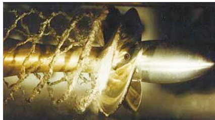
Propeller cavitation Image courtesy: http://www.rcboataholic.com/hardware/prop.htm
