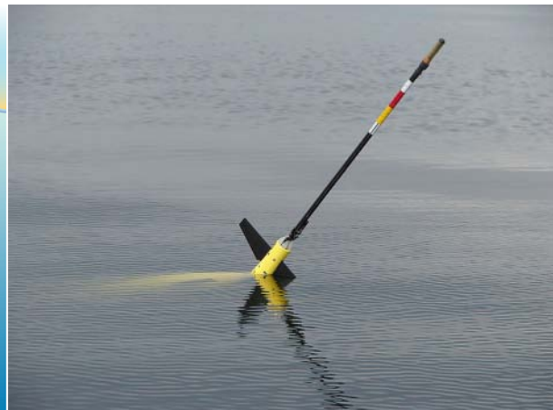
L: Sample dive profile of the Spray Glider, similar to those of other gliders as well (note compressed scale in graphic: actual is 1km dive, 5km horizontal range, in 10 hours) Image: WHOI R: Seaglider “phones home” at top of its dive Image: Wiki commons
